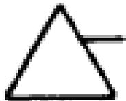
**TRANSFER OUT** – Indicates that this portion of the tree must be attached at the corresponding **TRANSFER IN**
