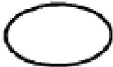
**CONDITIONING EVENT** – Specific conditions or restrictions that apply to any logic gate (used primarily with **PRIORITY AND** and **INHIBIT** gates)
