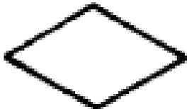
**UNDEVELOPED EVENT** – An event which is not further developed either because it is of insufficient consequence or because information is unavailable
