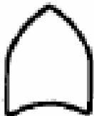
**OR** – Output fault occurs if at least one of the input faults occurs
